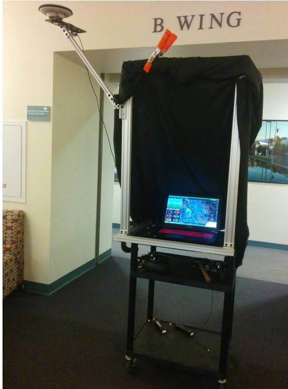
Figure 4.2: Our base station cart, from where we issue commands and monitor the system. It contains a Piksi RTK GPS connected to a NovaTel pinwheel antenna, a laptop computer, a telemetry radio for data communication, and a remote control radio for joystick control inputs.
