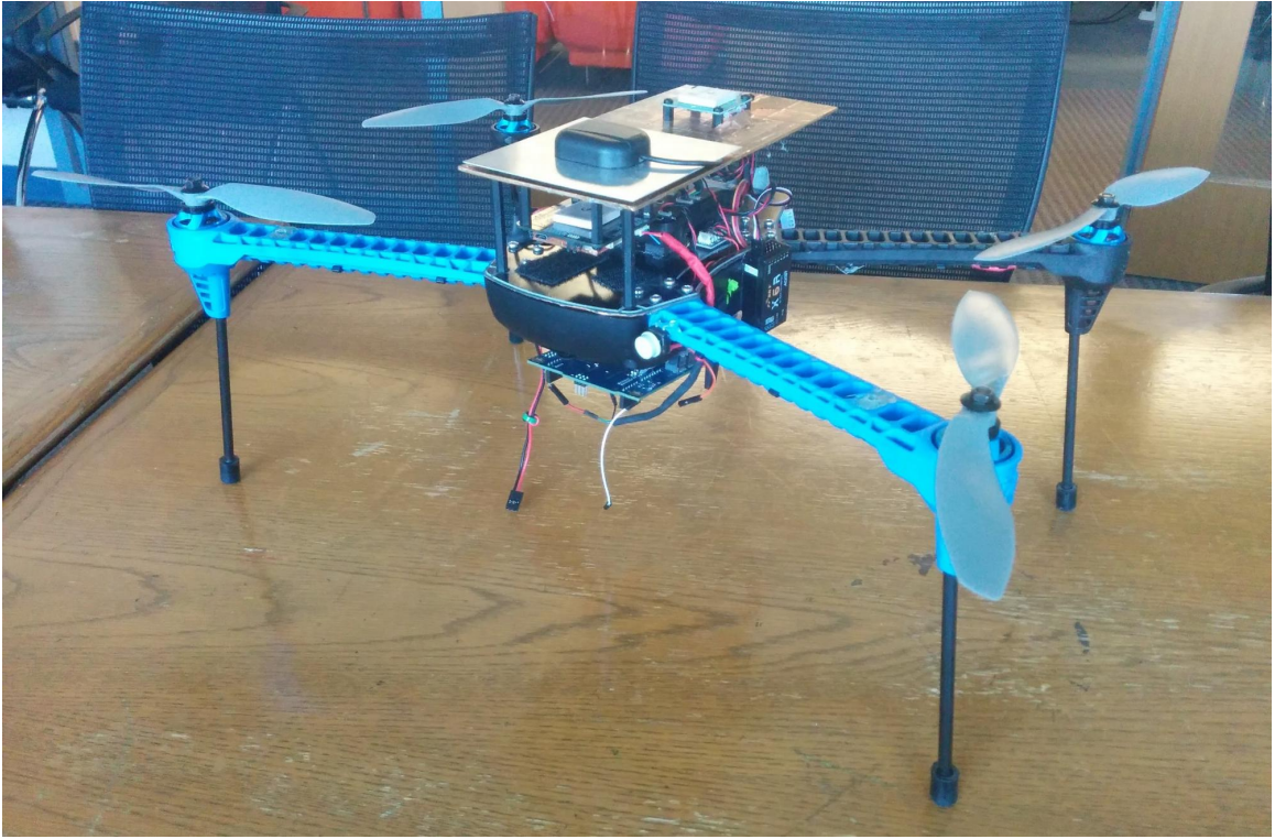
Figure 4.1: Our modified 3D Robotics Iris Quadrotor. A second platform on top of the quadrotor body holds a RTK GPS antenna and a conventional GPS module. This platform provides electromagnetic shielding between the sensitive GPS antennas and the rest of the quadrotor, as well as a clear sky-view during flight. An Intel Galileo companion computer is mounted on the underside of the body. The companion computer serves as an independent datalogger.
